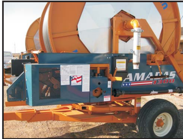
Easily Adjustable Speed Control with 2 Speed gearbox with 2 Step Pulley
