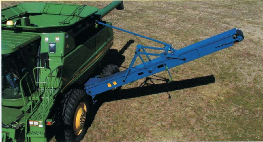
▲ Conveyor in extended position
