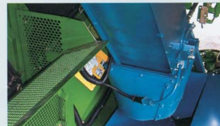
▲ Grain tank discharge spout gently feeds the unloading conveyor.
