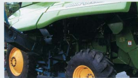
▲ Easy access is provided, as the conveyor system is designed not to interfere with the normal raising and lowering of the combine's side shields.
